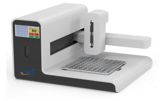
2.9.1 XYZ three-axis positioning, 100 sample positions, high-precision liquid injection pump
