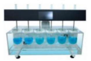
YKRC606 dissolution test instrument is a high-performance 6-cup 6-bar dissolution test device designed and manufactured strictly in accordance with the provisions of Chinese Pharmacopoeia and American Pharmacopoeia. It has high intelligence, advanced structure, accurate control and good reliability.
