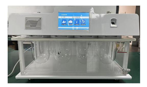
YKRC807 dissolution test instrument is a high-performance 8-cup 8-bar dissolution test device designed and manufactured strictly in accordance with the provisions of Chinese Pharmacopoeia and American Pharmacopoeia. It has high intelligence, advanced structure, accurate control and good reliability.
